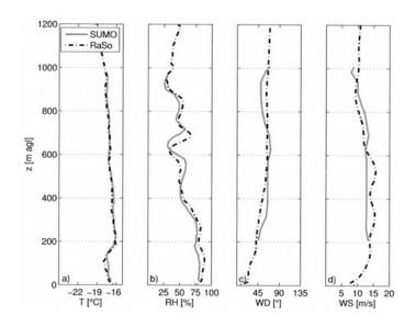
Figure 3: Direct comparison between the SUMO and RS- 92 radiosonde measurements (Figure 6 in Reuder et al (2009)).
